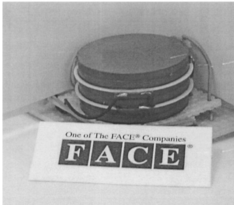
Fig. 8. Piezoelectric transformer, Transoner ® , operating in radial-extensional vibration mode.
